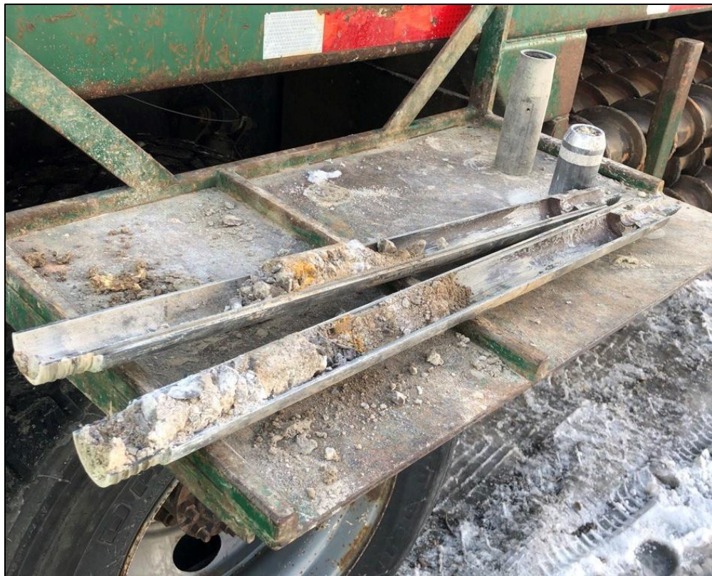
Figure 4: BH-3 Split spoon sample from 21.5' bgs
