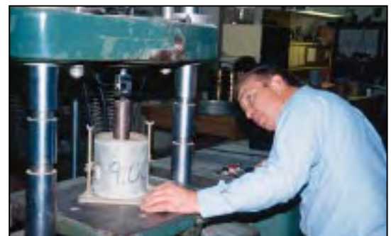
Figure 1. A technician applies load to a compacted soil specimen in a CBR mold. Specimens were loaded with and without sand layers to determine the effect of differing sand-layer thicknesses.
