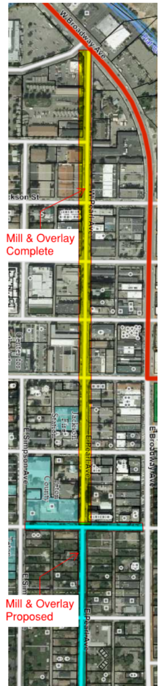
Figure 1 Showing resurfacing to date in Yellow and Proposed in blue.
