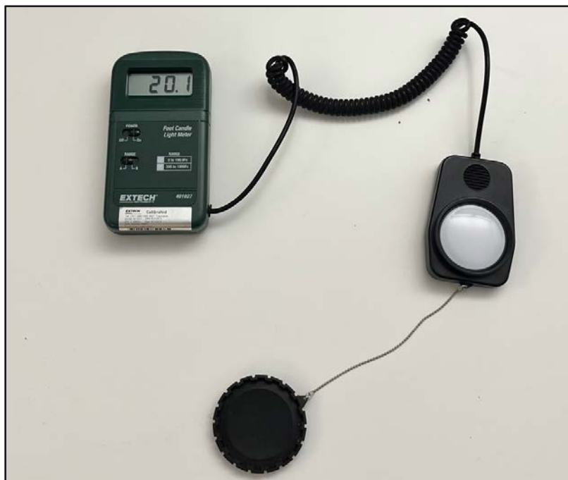
Figure 14 Sample Light Level Reading in Office Space
