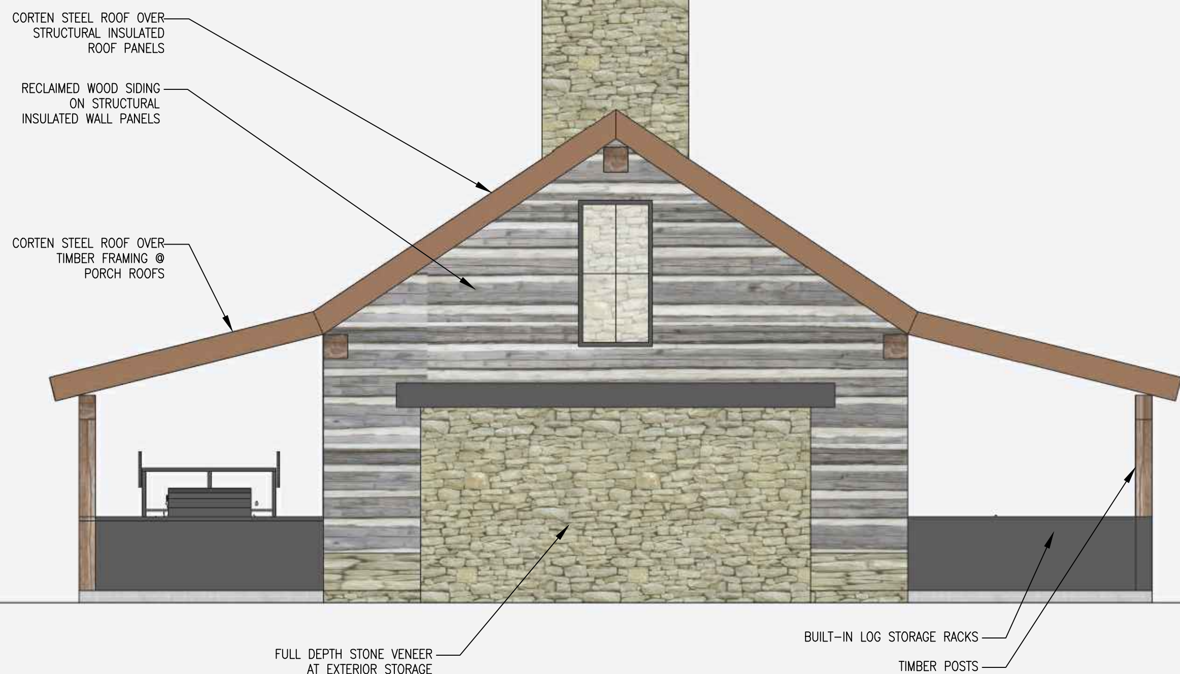
North Elevation - Fellowship Cabin ④ 1/4" = 1'-0"
