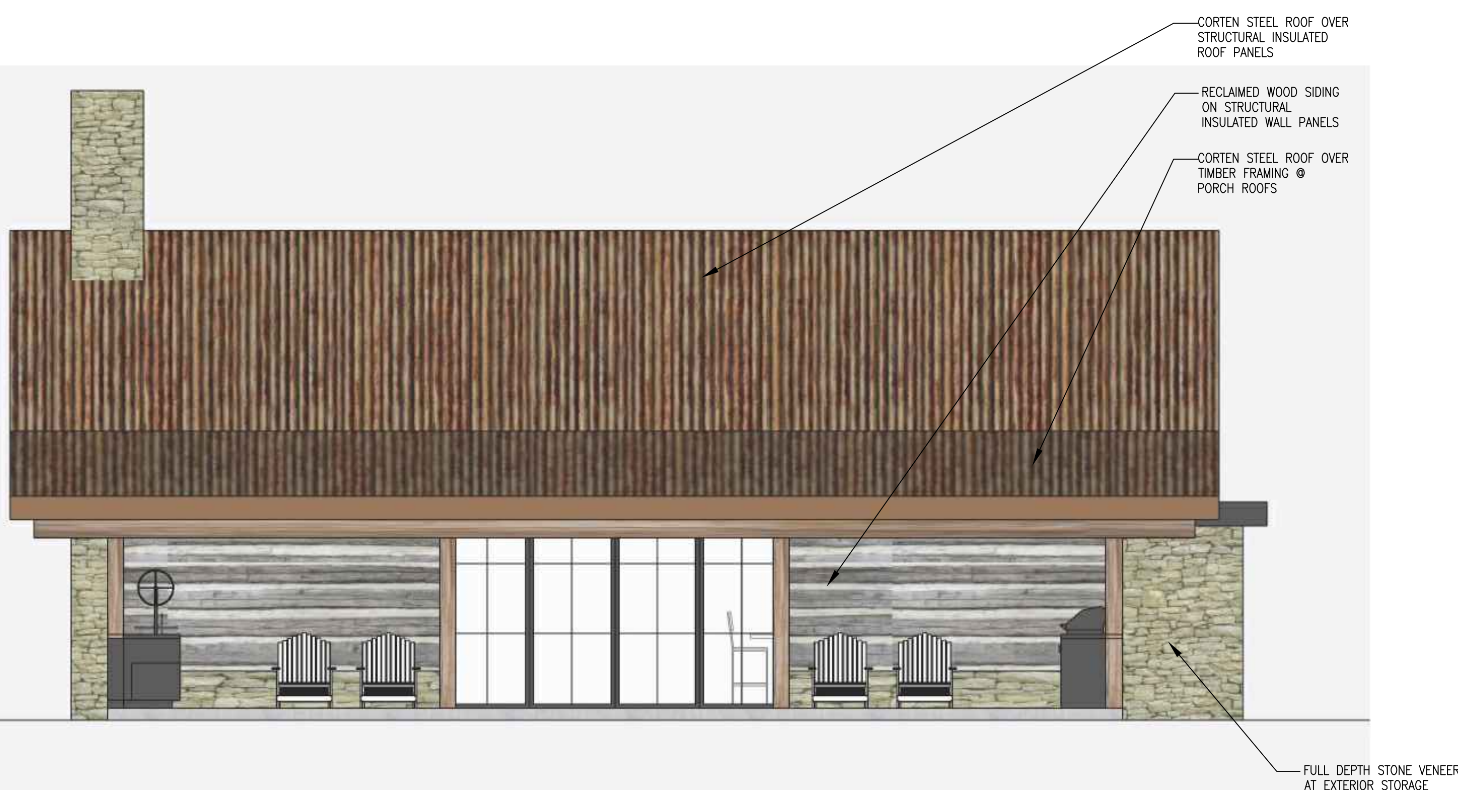
East Elevation - Fellowship Cabin ③ \frac{1}{4}" = 1'-0"
