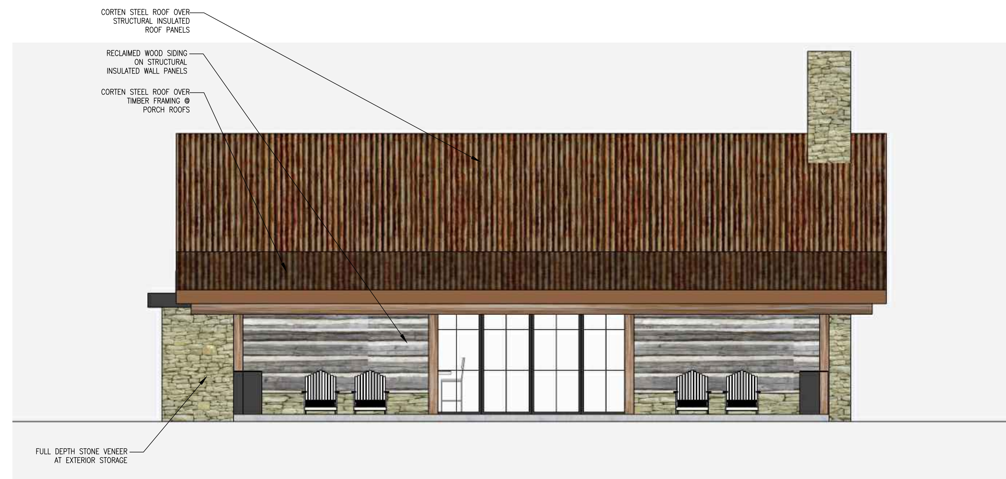
West Elevation - Fellowship Cabin ② 1/4" = 1'-0"
