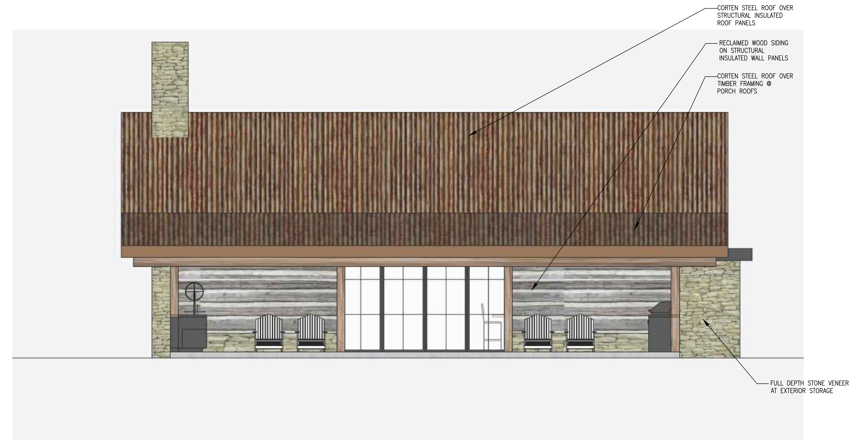
East Elevation - Fellowship Cabin ③ 1/4" = 1'-0"
