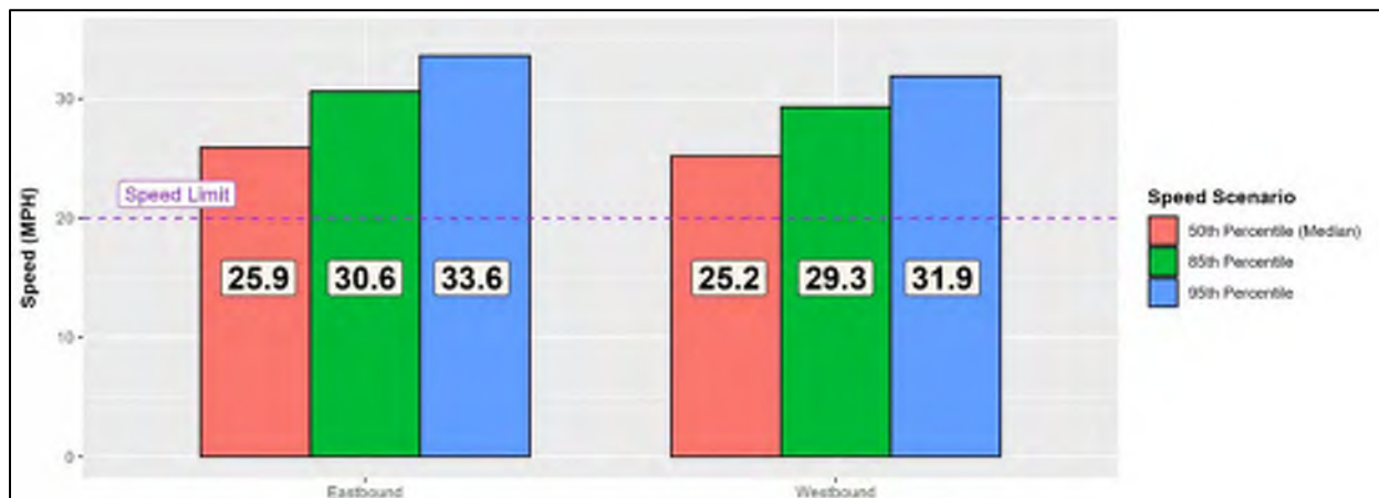
FIGURE 23: HIGH SCHOOL ROAD WEST OF GREGORY LANE POSTED SPEED LIMIT IS 20 MPH; 85TH PERCENTILE SPEED EXCEEDS 10 MPH HIGHER THAN THE POSTED SPEED.
