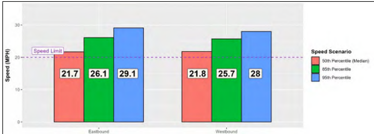
FIGURE 25: MIDDLE SCHOOL ROAD NORTH OF HIGH SCHOOL ROAD POSTED SPEED LIMIT IS 20 MPH; 85TH PERCENTILE SPEED IS WITHIN 10 MPH OF POSTED SPEED.
