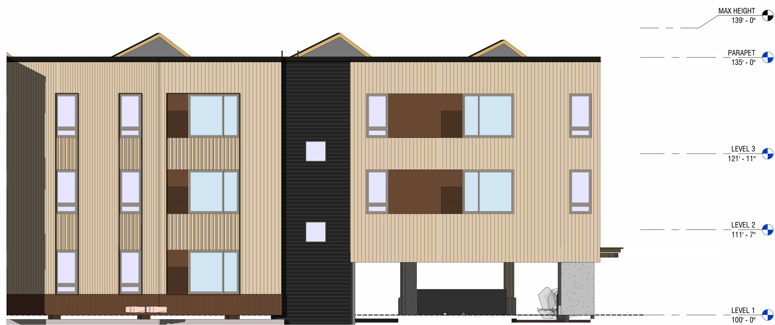
1 ELEVATION AT COURTYARD NORTH 1/8" = 1'-0"
