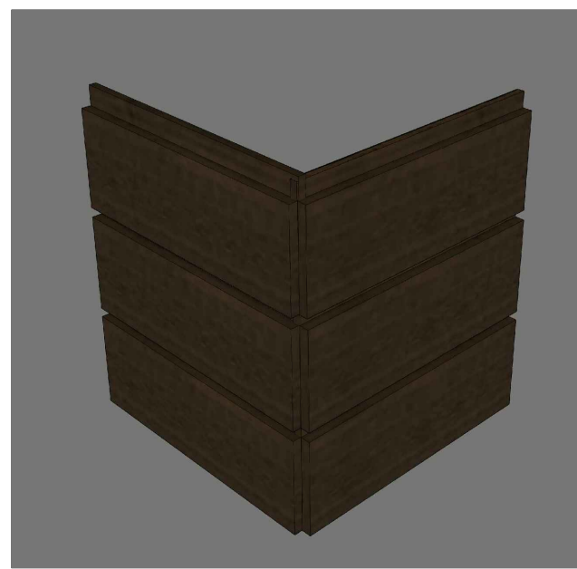
LINEWORK ONLY APPROX. PROPOSED COLOR 3X SHIPLAP SIDING, 11" APPROX. EXPOSURE, 1" REVEALS, QUIRK MITER CORNERS STAINED TO MATCH EXISTING CHURCH BLDG
