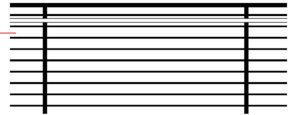
GUARD RAIL FABRICATED, 1.5" X 1.5" ANGLE FRAME AND BALUSTERS. 1/2" ROUND HORIZONTAL BARS. 1.5" ROUND HAND RAIL.
