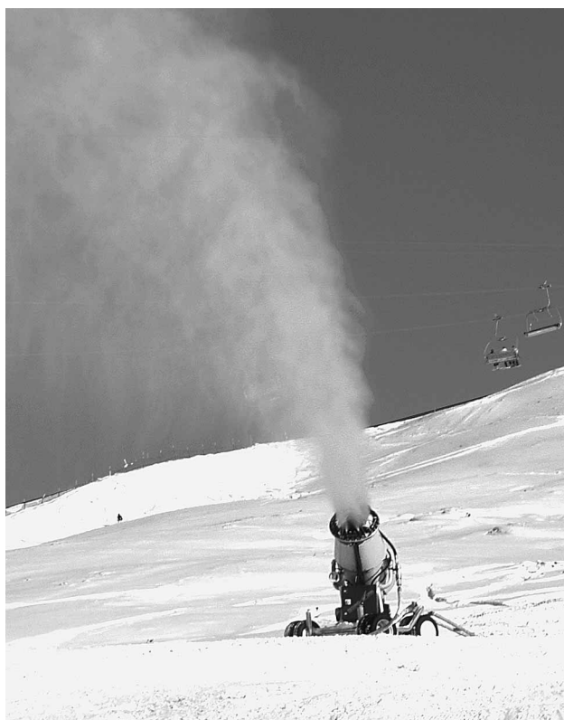
Fig. 2. Production of artificial snow. Water is atomised through nozzles of snow machines into droplets and blown into the air with a built-in fan or with high pressure. The droplets usually require temperatures of below -7^{\circ}\text{C} in order to be frozen thoroughly when they fall to the ground as snow.
